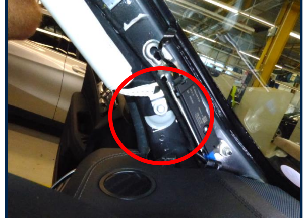
Bodyshell holes sealed
