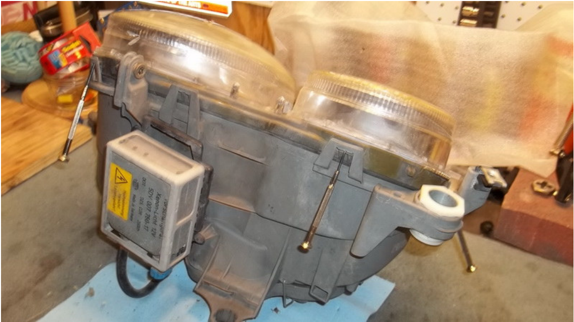
Very carefully release tabs using screwdrivers. Work slowly and, as multiple tabs are released, begin to separate the lens assembly from the housing.
