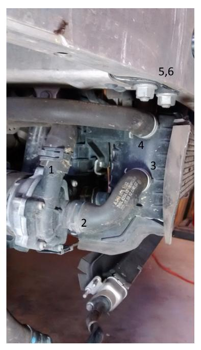
1-4: Remove clamps with water pump pliers.
