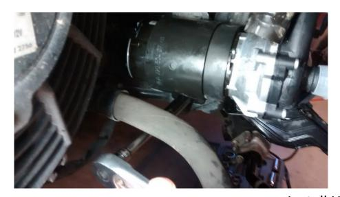
Install new I/C pump. One nut.
