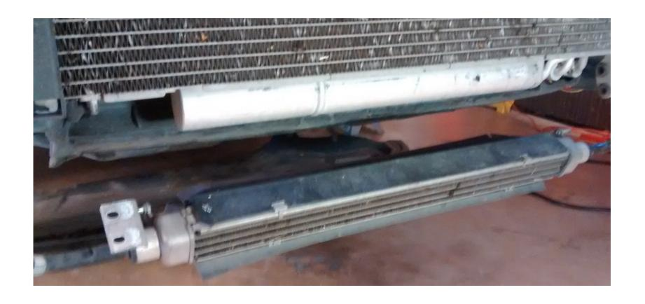
Remove two nuts on left side, bracket pulls off and cooler slides out of other mount to release from heat exchanger.
