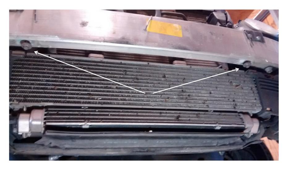
These are the two bolts referenced in picture 1 of the MB document. Front under-tray must be removed, bumper lip pulled forward, and 12" extension to reach these 10mm hex head bolts. (Photo obviously taken after bumper removed.)
