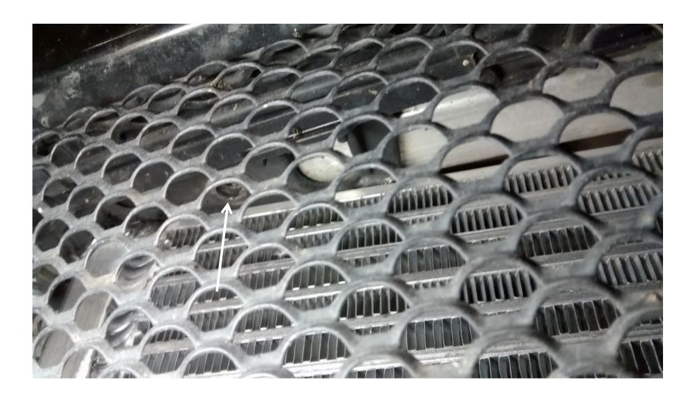
This is the interference point. 10mm hex head bolt screws into location shown by arrow. You can reach it by pulling out the lower lip of the bumper while pushing in at the tab location to thread the bolt into the frame. Challenging but not impossible.
