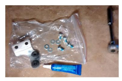
Transfer grommets from OEM brackets to aftermarket brackets, Loc-Tite or equivalent, mount the cooler to the HF.
