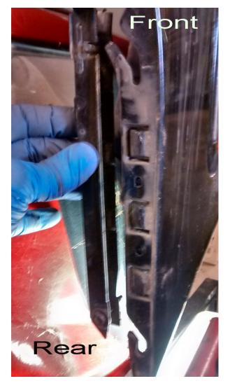
These hold on your bumper. The terminal strips are tight and dirt makes them difficult to remove. You may need to lightly tap them forward with a small hammer to break them loose. To reinstall place front pin in front slot, push strip onto the fender/bumper interface, them pull them towards the rear of the car (this may take some effort).
