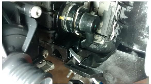
Use a small screwdriver to release the heat exchanger from the lower brackets. Left-hand photo is of driver's side, above photo is of passenger side. Press up from underneath to release. Pull heat exchanger out and down to remove.
