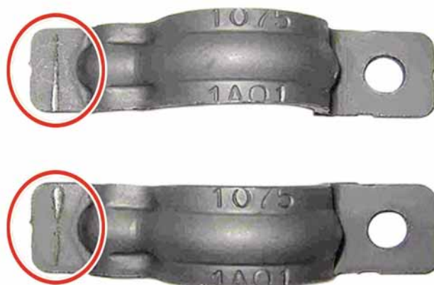
Cushion frame bracket with signs of wear
