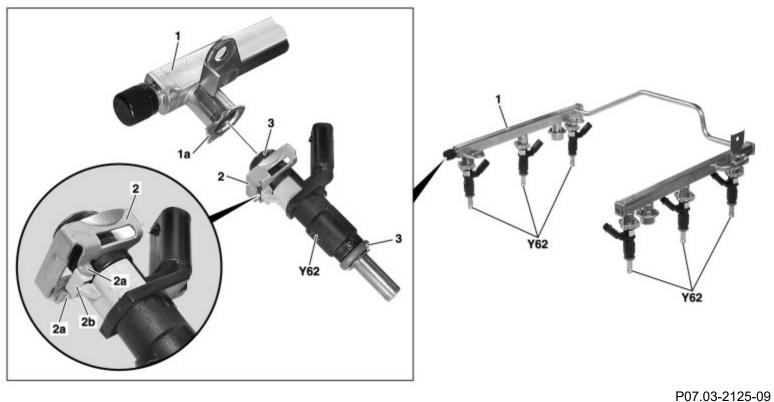
1 Fuel rail 1a Connection 2 Securing clamp 2a Pins 2b Molding 3 O-ring
