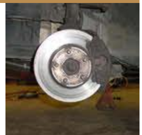
Damaged brake rotor from metal-to-metal contact
