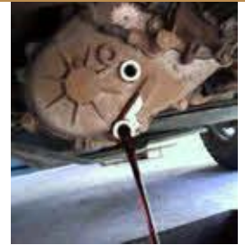
Draining the old transfer case fluid
