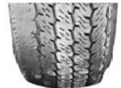
Signs of irregular tire wear
