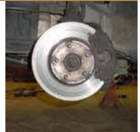
Scored and damaged brake rotor
