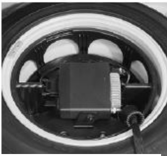
E-Class, radio mount in Vito, loading space /Spare wheel well, Code 335 1)
