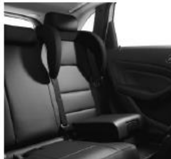
B-Class, rear bench seat with integrated child seats, Code 248
