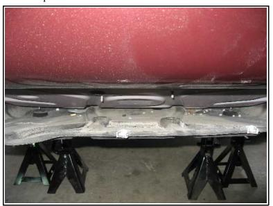
(12) You need to cut out some plastic off of the black trunk cover in order to allow clearance for the hitch. The hitch instructions said to cut out this area (see pic below)
