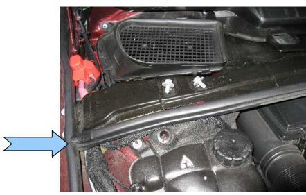
**Step 5:** Now remove the cross brace by grabbing it in the middle and pulling straight out and up at the same time.
