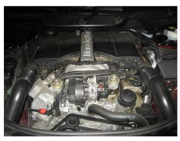
**Step 7:** Remove the two air tubes connected to the air filter boxes. You just need to pull them back in order to separate them from each other.
