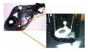
A knocking noise that occurs when the power window is operated downward and reaches the lower limit position may be caused by a broken plastic limit stop. To remedy, perform the following.
