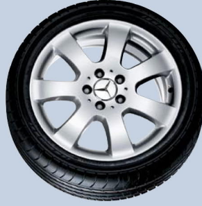
17 7-SPOKE WHEEL 7.5 J x 17 ET 56 · 235/65 R17 B6 647 4247 * Titanium silver finish; 17" wheels are exclusively compatible with 6-cylinder engines. For 8-cylinder vehicles at least 18" are required
