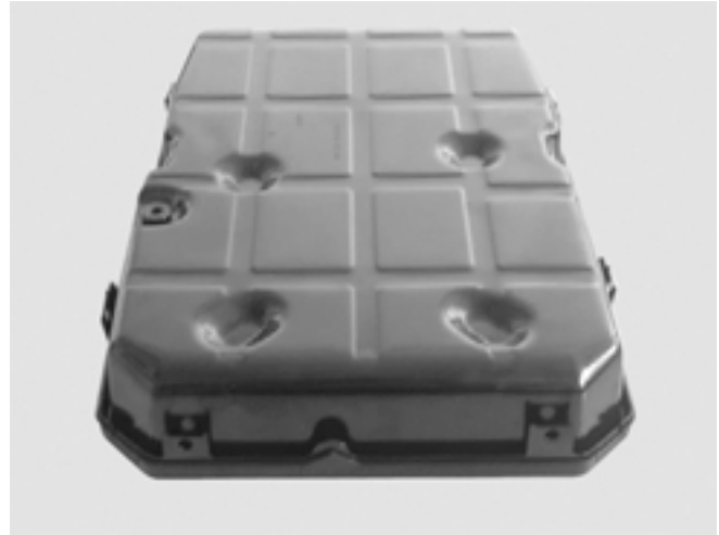
Figure 2. Oil pan (with oval forms) transmissions 722.9 as of production date June 21, 2010. P00-40-2028-01
