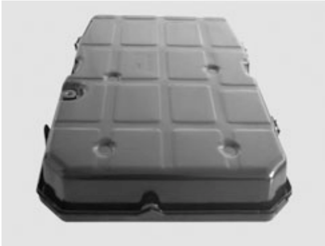
Figure 1. Oil pan (with round forms) transmissions 722.9 up to production date June 21, 2010 P00-40-2027-01
