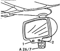
That's not all, folks. You can also check to see whether the transmitter sends a signal using an IR Signal Indicator Card (like Radio Shack 276-0099). Follow the instructions that come with the card. The Mercedes-Benz Diagnostic Manual outlines the procedure to determine whether the vehicle then correctly reads the signal.
