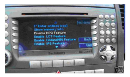
Using the arrow keys, highlight the MP3 feature and enable it using the "OK" button.
