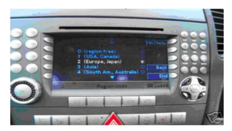
Using the arrow keys, highlight the region free setting and enable it using the "OK" button.
