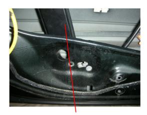
Step 7: Becareful the unit can fall if you remove all of the screws. Push back the window bracket to remove the unit.
