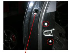
Remove screws. 3 on the door. Unscrew the key sensor ( Up to the guide/ Screw catch) and remove the sensor.
