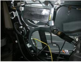
Step 3: Remove the Foam paneling / covering. No need too remove it completely. Start from the back of the door. You need only to fold it half way and tack it to the front (fold it over).
