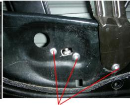
Drill out the rivets
