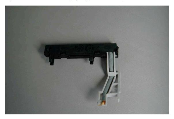
10. The front and rear door modules are the same, but they are different left to right. The part number for the right side A 220 820 04 21; the left is A 220 820 03 21 (and it has a large "L" above the bar code on its label, and another on the gray LED support). The right one has "R"s.
