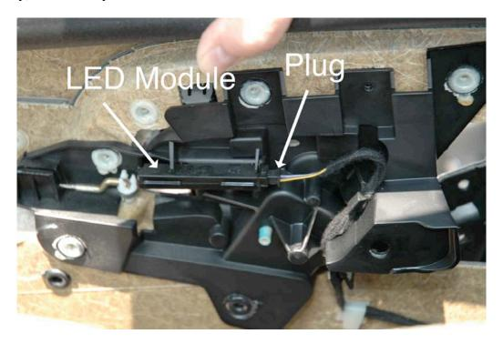
The clips on a new module can be seen projecting downward in the photo below.
