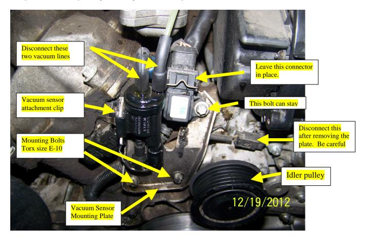
There is an electrical connector just to the right of the vacuum sensor mounting plate right above the idler pulley that will be in your way when you try to remove the water pump. After removing the plate carefully disconnect this and move the wire out of the way.
