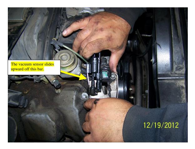
Now you can swing all of the released components up and out of the way.
