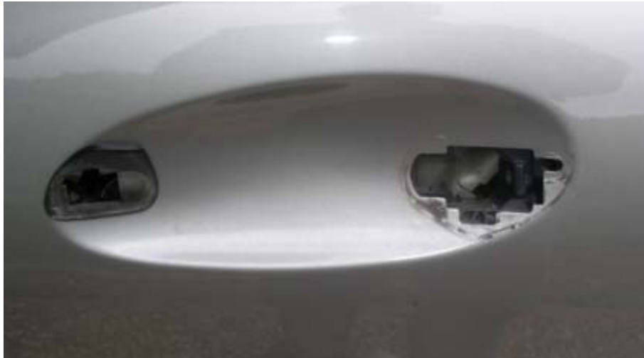
Figure 11 Two Torx Screws Removed.
