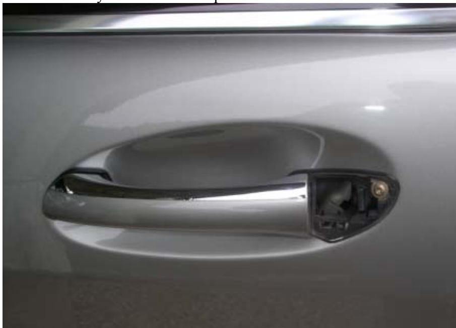
Figure 9 First Part of Rear Door Handle Removed
