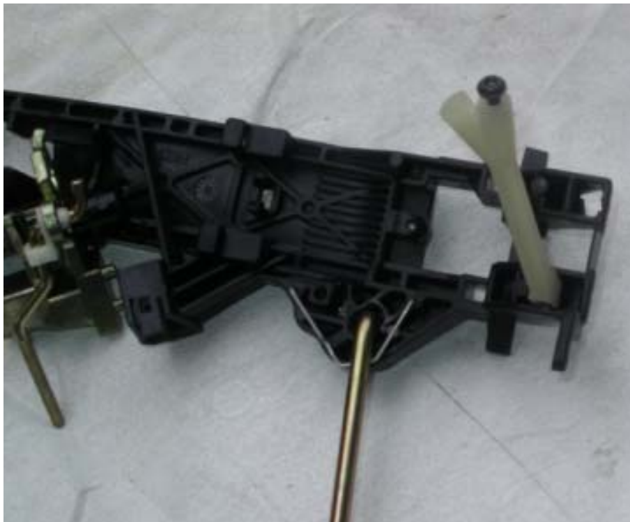
Figure 15 White 'Y' Bracket Mounted on the Door Handle Mechanism
