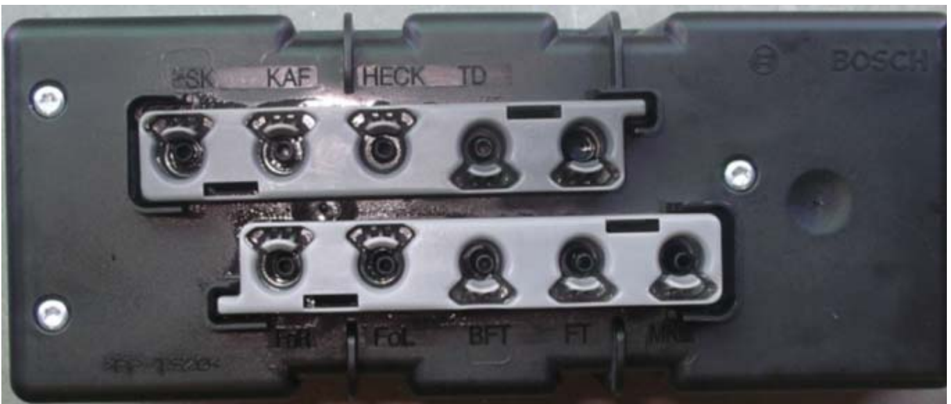
Figure 2 PSE Pump Air Line Port Designations
