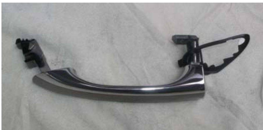
Figure 10 Second Part of Rear Door Handle Removed
