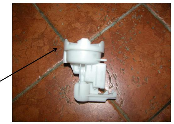
You can see here that the cap has sheared. Drilled these two rivets out.
