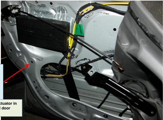
Once everything is in the proper position you can insert the other two screws on the edge of the door that holds the actuator. Don't forget to tighten this screw. They are all **T20 Torx**.
