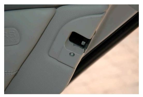
7. You may remove the plugs from the back of Door Control Module (DCM) on the upper panel that you removed, if you wish. It is not absolutely necessary, but it does provide a bit more room to move the panel; it also disables the window. The plugs will only go back one way (they are keyed) so there is no need to mark them. I did not unplug the tweeter that is in the panel. If you are removing the DCM, it is held to the panel by four plastic spring clips and comes out easily.
