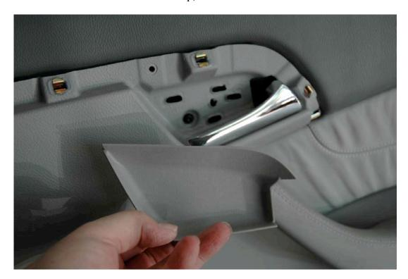
4. Then, using a wedge or a small, dull knife, pry the plastic panel out. On my door it was not necessary to remove the two silver #20 Torx bolts holding the upper door grip in place, but you must remove the black #30 Torx bolt in the plastic housing for the door handle (leftmost white arrow). The clips for the LED module will be visible; you may have to remove silicone used to keep the clips in place.
