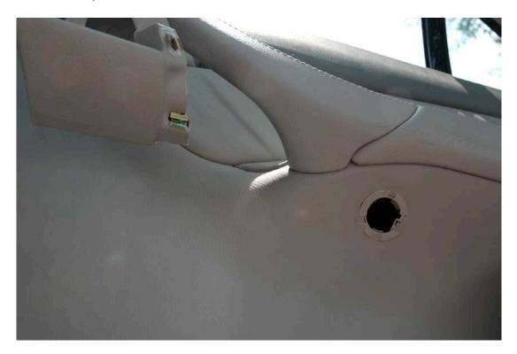
6. Then, remove the plastic trim around the door closure mechanism, below – it is held in place by a single #20 Torx screw. Note the small plastic clip on the back side of the trim piece that must fit under the side panel when you replace it.
