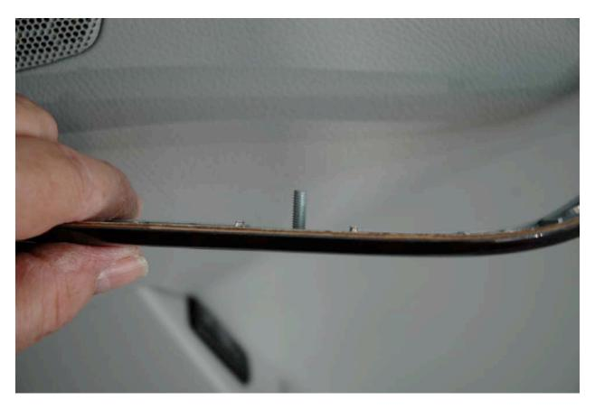
2. The wood trim is held in place by bolts welded to the metal backing of the wood itself, as shown above. It is fairly sturdy. The bolts fit into the slots visible in the photo below. After the trim is removed, unscrew the 2 black bolts (#20 Torx) visible in the photo below.
