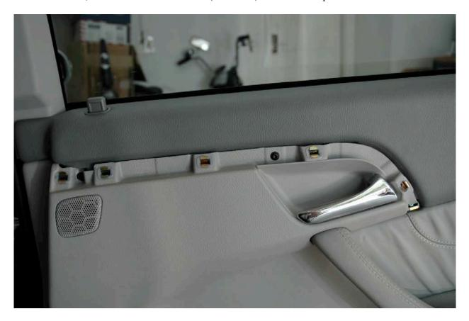
3. Once the wood trim is removed, use a small blade to remove the cup behind the inner door handle. It just pries out either from the top or the side toward the front of the car. Then, remove the third #20 Torx bolt located behind the cup, visible above the inner door handle.
