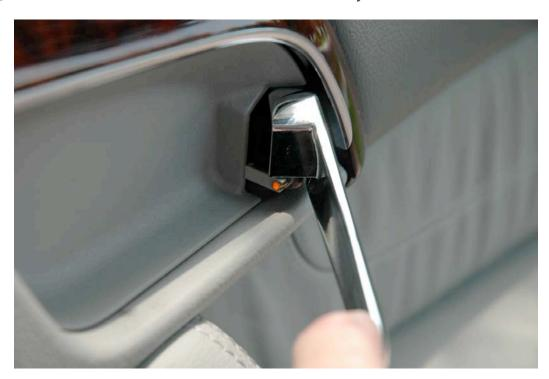
13. When you removed the door panel, one or more metal clips may have fallen off of the panel, toward the rear. Here's where they go, as you start to reassemble the door. The narrowest edge of the clips goes over the metal edge that runs below the weather strip of the stationary window.
