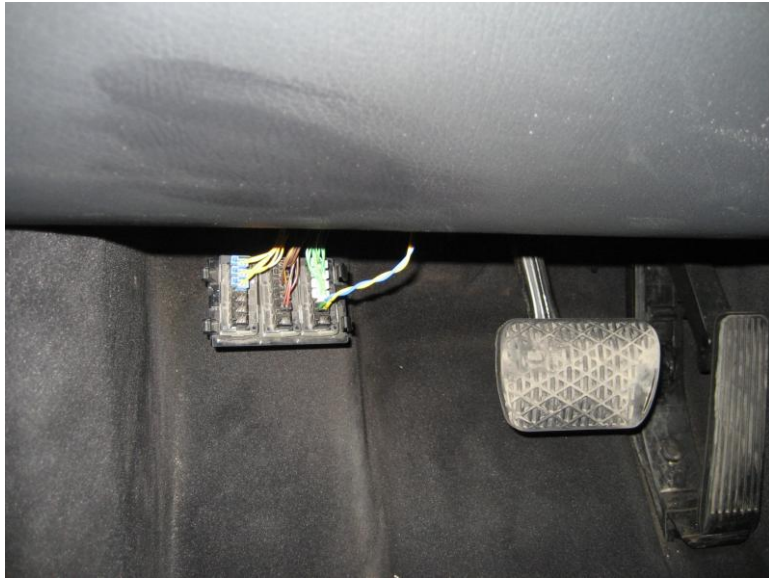
Pic. 2 Location of Chassis CAN Voltage Distributor Connector
