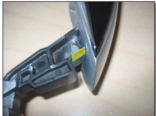
Figure 2 - Front rib beveled 45° P-B-72.00/85
