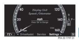
▶ Press button OK again if you would like to change the current status. Depending on the previous status, the Display Unit Speed-/Odometer will be switched to miles or km.
