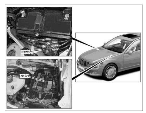
Location in engine compartment, shown on model 221.095
