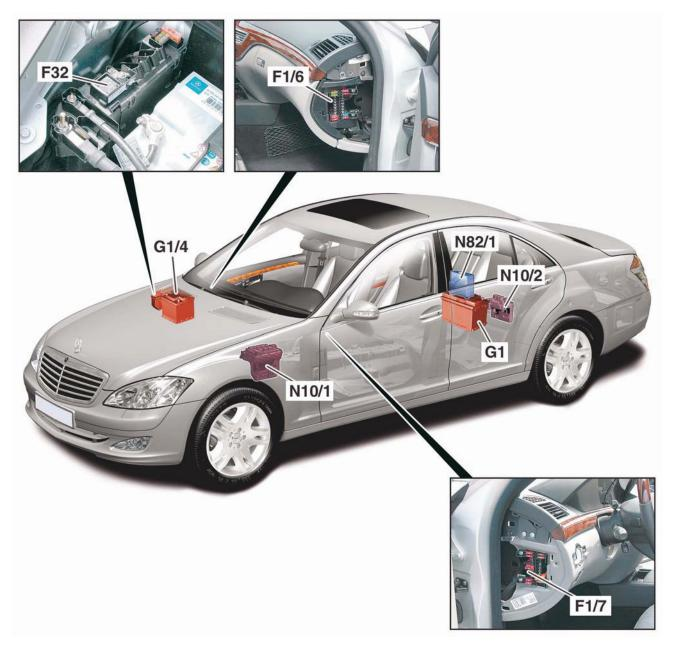
F1/6 Right instrument panel fuse box F1/7 Left instrument panel fuse box
