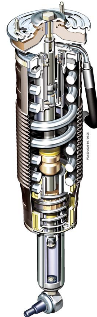
Federbein Vorderachse ABC-Federungssystem (Active Body Control) S-Klasse (BR221)
