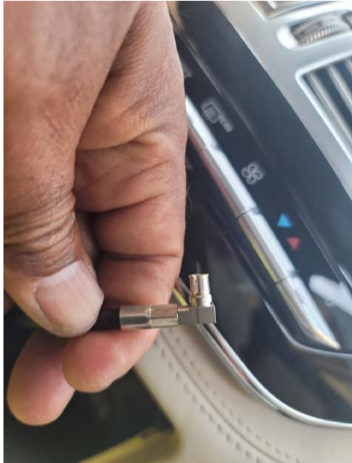
The removed cable should look like this.
