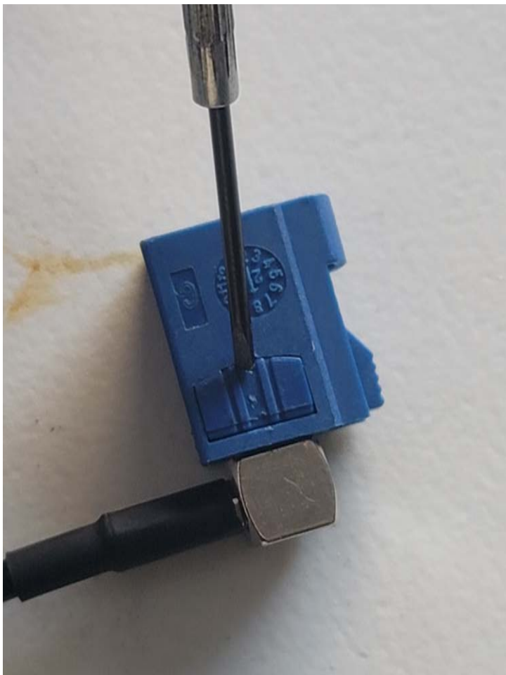
Take the Blue FEMALE FAKRA cable. Depin the unit by lifting out the blue retaining clip.
