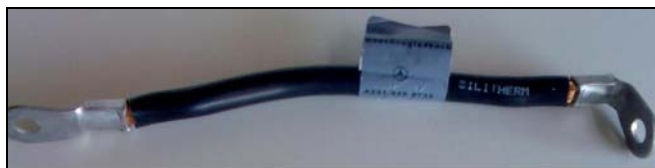
Figure 2 P-B-54.18/209 Incorrect ground strap
