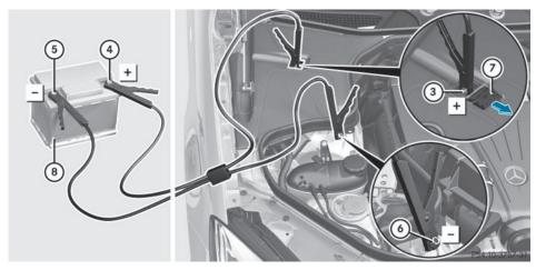
Position number (8) identifies the charged battery of the other vehicle or an equivalent jump-starting device.
