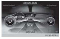
By setting the climate mode, you determine the strength of the airflow based on the air distribution set. The setting is only active when the air-conditioning system is set to "AUTO".
