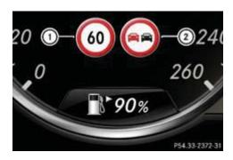
A maximum permitted speed of 60 km/h (60 mph) 1 and an overtaking restriction 2 apply.
