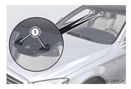
Traffic Sign Assist displays the maximum speed permitted and overtaking restrictions to the driver in the instrument cluster. Driving onto a section of road in the wrong direction triggers a warning. Traffic Sign Assist detects traffic signs with camera system ① attached behind the top of the windscreen. The data and general traffic regulations stored in the navigation system are also used to determine the current speed limit.
