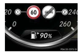
A maximum permitted speed of 60 km/h (60 mph) ① applies. The overtaking restriction no longer applies ②. The crossed-out no overtaking traffic sign is displayed for five seconds.
