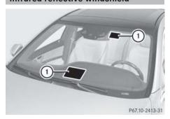
The infrared reflecting glass prevents the vehicle interior from becoming too hot. It also blocks radio waves up into the gigahertz range.
