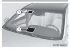
The infrared reflecting glass prevents the vehicle interior from becoming too hot. It also blocks radio waves from penetrating the windshield up into the gigahertz range.
