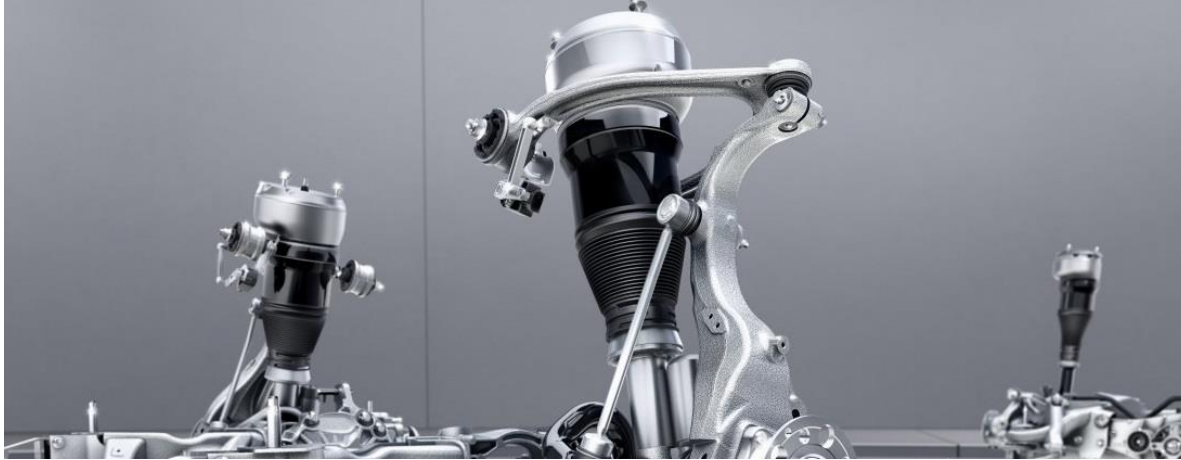
AMG Sport Suspension based on AIRMATIC Standard on S63
