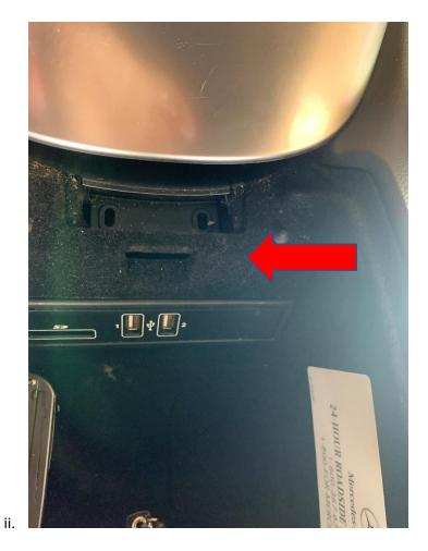
b. Use a plastic interior molding tool to pry open the upper leather panel. Don't use a sharp pick for this.
