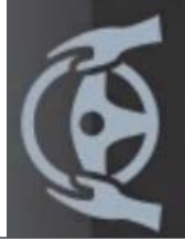
Active Steering Assist switches on but is not ready for steering intervention (passive, icon gray)
