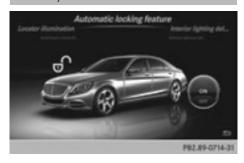
When the automatic locking feature is activated, the vehicle is locked automatically when the ignition is switched on and the vehicle is traveling faster than walking pace.
