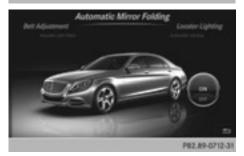
When the Automatic Mirror Folding function is activated, the exterior mirrors fold in automatically as soon as you lock the vehicle from the outside. The exterior mirrors fold out
