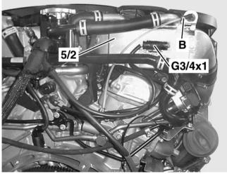
To test the "divert air" function a test connection (B) has been provided on the charge air cooler on the right-hand side of the engine (5/2), in the area of the  $O_2$  sensor connection at the right upstream of the TWC (G3/4x1).
