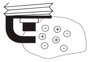
After end of sparking, a test voltage of 1 kV (resulting from 23 V auxiliary voltage) is applied to the spark plugs between the center and ground electrodes.
