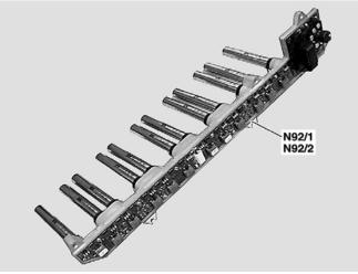
The required ignition voltage is built up significantly faster using the ECI ignition system. Here a pilot control of the ignition coil (building up and removing the magnetic field) is no longer required.
