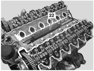
The vacuum pressure required for actuation is provided from a vacuum tank (22), which is located in the "V" of the crankcase instead of the oil-water heat exchanger.
