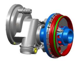
At a specific vacuum (> 50 mbar) in the charge air manifold the connection to the crankcase is sealed by means of a diaphragm in the pressure regulator valve.
