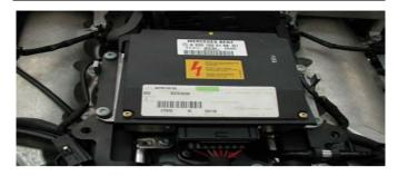
The power supply unit operates as a DC voltage supplier, the function of which could be compared to that of a power station.
