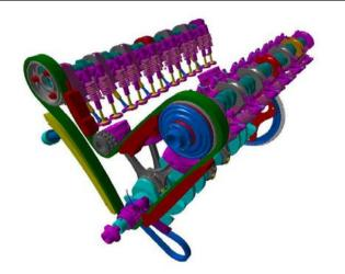
Camshaft drive ensues from the crankshaft by means of a twin roller chain. A sprocket wheel is used in the V-center for deflection purposes. Otherwise the chain is routed through slightly bent slide rails. The chain tensioning force is achieved over a tensioning rail by means of a hydraulic chain tensioner.
