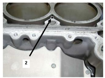
The cylinder liners are made up of an alloy of aluminum-silicon (silitec). They have a wall thickness of 2.5 mm.
