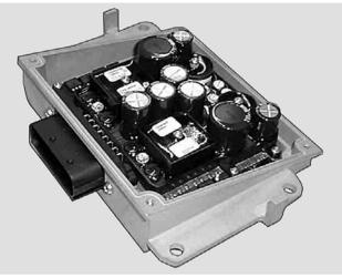
The power supply unit consists of a housing made of light alloy, in which several electronic components are accommodated. These electronic elements are available in duplicate for each cylinder bank.
