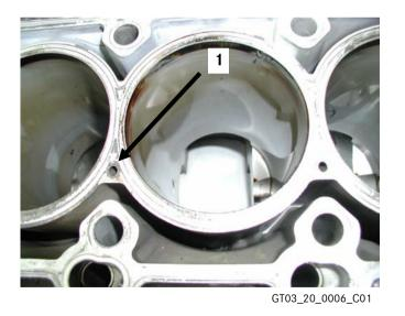
In order to do justice to the higher heat and pressure loads, the wall between the cylinders of the upper crankcase section have been widened compared with the M137 by 2 mm to 8 mm and in each case 3 water cooling bores (1 and 2) have been integrated into the walls.
