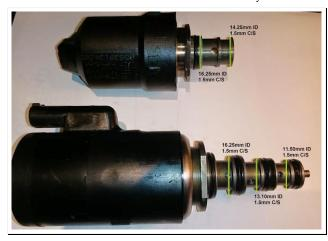
The main control valves (y1,y3 in schematic, lower valve in picture) is a 3-position valve. In the outer position it allows fluid to enter the strut, in its center position it closes off the strut, and in the inner position it allows fluid to leave the strut. When the ABC system is active, this valve is doing all the work.
