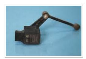
In each wheel well you find a ride height sensor. It reports to the ABC control module how high the corner of the car is. If a corner of the car gets too low, an "ABC Car Too Low" message will appear on the dash.
