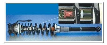
Imbedded inside each strut is an electronic sensor that measures how far extended the strut is. It reports this to the ABC control module. The control module uses this information along with other sensor inputs to decide how much fluid it wants in the strut.
