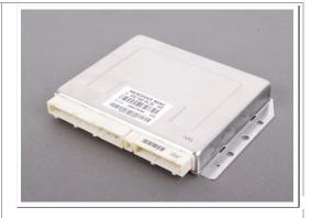
If the control module senses inadequate pressure to operate, or if any of the sensors provide in-plausible data, the system will shut itself down for safety reasons. The offending sensor will be logged for later retrieval by the SDS system.
