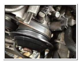
The power steering and ABC pump are integrated into one unit, referred to as a Tandem Pump. Although the two pumps share the same housing, they are separate components otherwise. It is possible for the ABC portion of the pump to fail but the power steering portion of the pump is fine (and vice versa). But if one portion fails, both have to be replaced since they are one unit.
