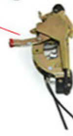
Left Rear Lock Cylinder (Shown With Lock Used in Model years '90-'94) P/N 1298002172 (or 1298000072 in some models)
