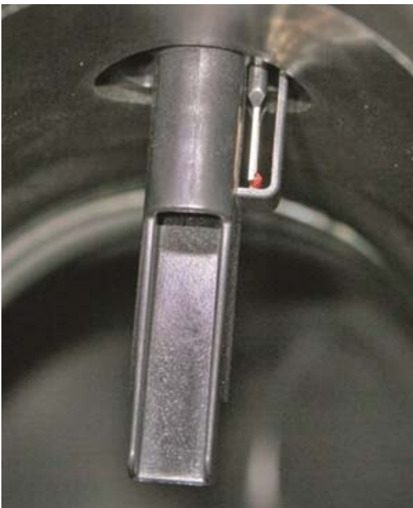
o This MAF sensor is mounted in the top of the air filter housing. Notice the IAT sensor on the right; it's part of the MAF assembly but it is not used for measuring airflow.
