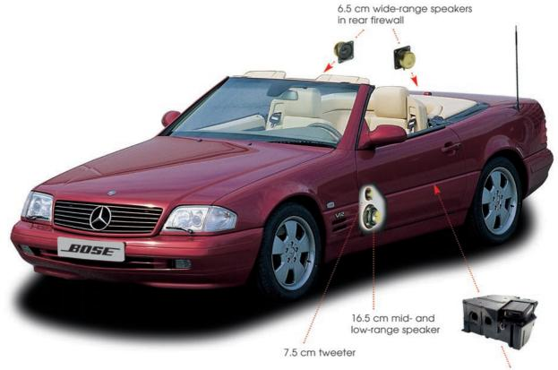
System Electronics and 13 cm low frequency transducer in a tuned, ported enclosure (volume 12 I) applying the Acoustimass® technology under storage Lid hind left seat
