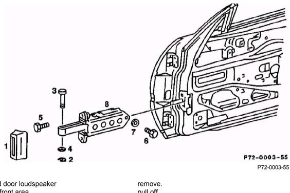
Air duct and door loudspeaker Door foil in front area Seal (1) over bolt Lock (2) on bolt Bolt (3)
