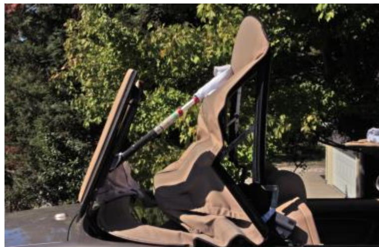
Top position for bow cylinder top pin e-clip, wave washer and wire guide removal/installation. For pin removal see next picture, top must be moved forward some. Easier to remove e-clip, wave washer and switch guide in this more vertical position. Note the high-tech paint extension handle to brace soft top.
