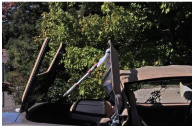
Position for bow cylinder bottom pin, e-clips(2) and pin removal/installation, switch removal/install and main top pin removal/install. Top raised but not latched in front, bow up. Rolled towels to cushion and prevent top from latching in front.
