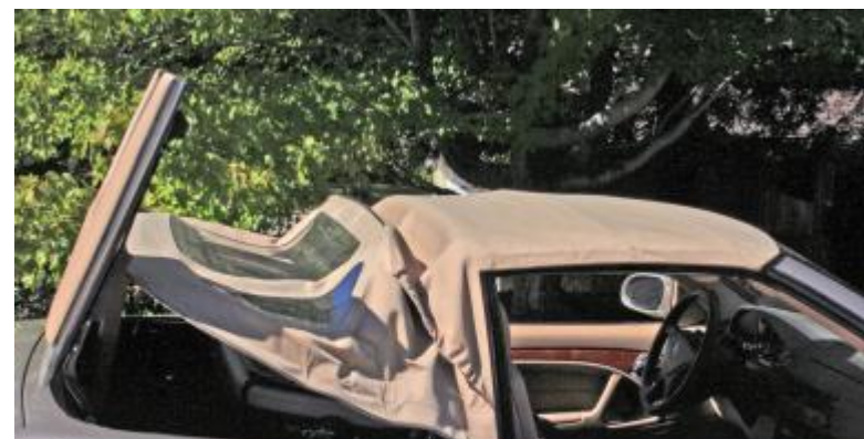
Position for bow cylinder removal from within the top frame after pivot pins, switch and hydraulic lines are removed/disconnected. Top raised and does not need to be latched, just the only picture I have in this position.
