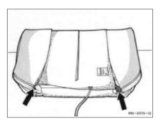
10 Install seat cushion cover so that electric wire passes through punched hole in rubber/hair pad (arrow).
