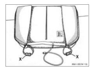
9 Wrap plug connectors in upholstery padding and insert into tacking channels.
