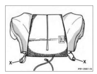
19 Wrap plug connectors with upholstery padding and insert into tacking channels (arrows).
