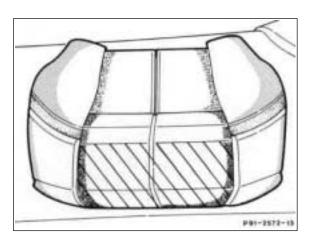
7 Position heating pads (2) for seat cushion on rubber/hair mat with felt side pointing up, align and cement on at front.
