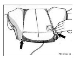
20 Install backrest cover; pass connection cable for heater pad through rubber/hair mat at bottom (arrow).
