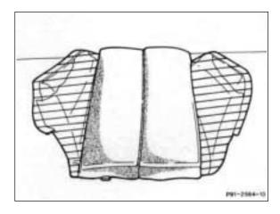
16 Position heating pads (5 and 6) for sides with textile side (heat conductor) pointing up and cement to rubber/hair pad in correct position.
