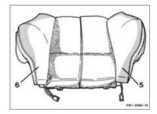
17 Position heating pads for backrest upholstery with felt side pointing up, align and cement onto rubber/hair pad at top (shaded area).
