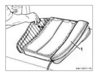
6 Coat front of rubber/hair pad (shaded area) with cement.
