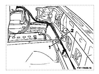
20 Lay pneumatic line (item 2, 4800 mm long) for orthopedic driver's backrest in line duct on left rear side section and left floor; where applicable lay pneumatic line (2670 mm long) for orthopedic passenger backrest in line duct on right rear side section and right floor.
