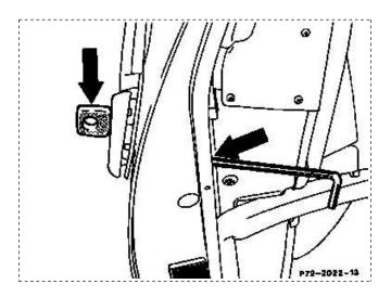
After tightening door handle check the small clearance between door handle and actuating lever for door catch, adjust if required.
