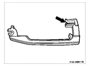
Insert lock cylinder into turning nut on door catch with turning rod; for this purpose turn lock cylinder 90° and fasten (arrows).
