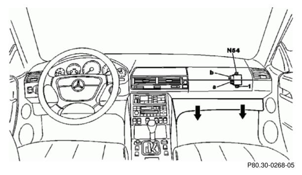
N54 Infrared remote central locking control module (IRCL), locations reversed on vehicles with right-hand steering
